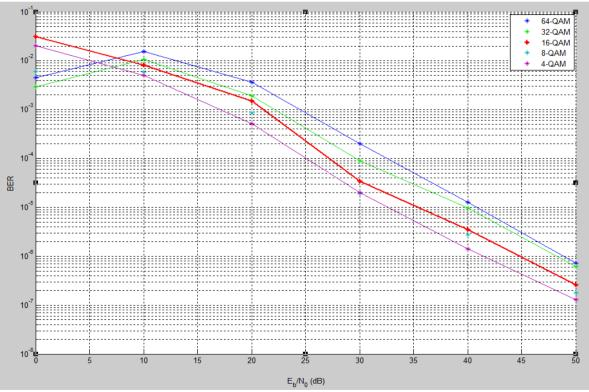
Figure 6 BER versus Signal to Noise Ratio for RFID System with M-Ary QAM modulation in Rayleigh Fading Channel
