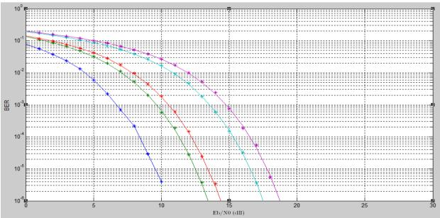
Figure 4 BER versus Signal to Noise Ratio for RFID System with M-Ary QAM modulation in AWGN Channel
