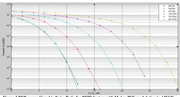
Figure 3 BER versus Signal to Noise Ratio for RFID System with M-Ary PSK modulation in AWGN Channel
